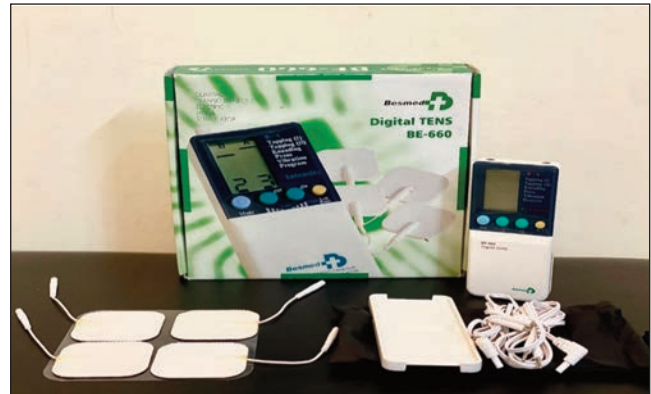
Figure: The transcutaneous electrical nerve stimulation (TENS) machine used in the study.
